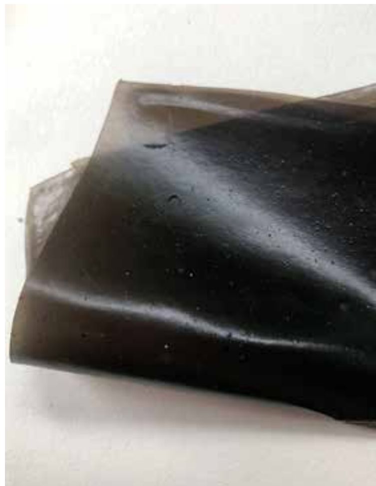
Bioplastic made of furcellaran, that is extracted from local seaweed ( Furcellaria Lumbricalis ). The material is dyed with burnt seaweed and cephalopods ink that is primarily composed of melanin. Experiment by Kärt Ojavee (2020)
