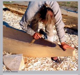
The Estonian dugout canoe, or one-log boat, has been used on Estonian inland waters for thousands of years. The body is carved from one aspen log. The boat is then placed on an oblong coal fire to stretch it with hot water and willow sticks. In the pictures, the canoe is being built and tested by students of native construction at the Viljandi Culture Academy.
